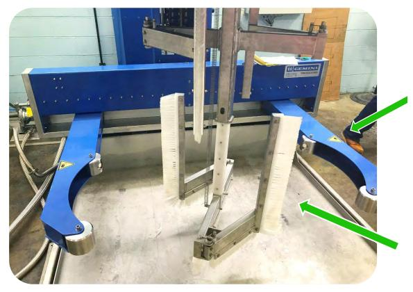
Lock-up vessel clamping device
